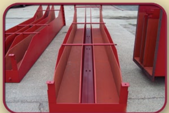
Rubber lined sand chute
